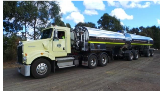
B-double, 7-axle, 19m (50.5 tonnes, PBS level 1) Av. net load 30,312 litres (25% of national fleet)
