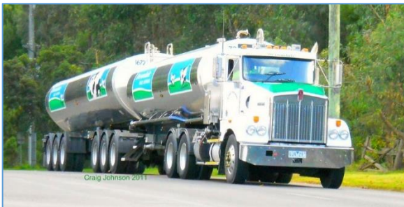
B-double, 9-axle, 25/26m (68.5 tonnes, PBS 2A) Av. net load: 36,169 litres (9% of national fleet)
