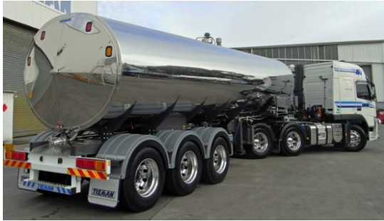
6-axle articulated, 19m (50.5 tonnes, PBS level 1) Av. net load 25,327 litres (50% of national fleet).
