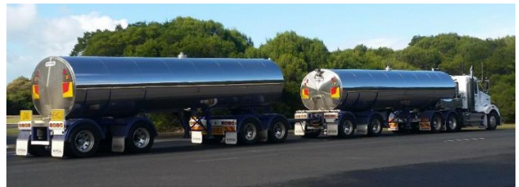
PBS 26m A-double (68.5 tonnes, PBS 2A) Av. net load: 38,296 litres (8% of national fleet)
