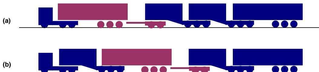
Figure 12. (a) ABB-quad and (b) BAB-quad vehicle configurations (Type II road trains)
