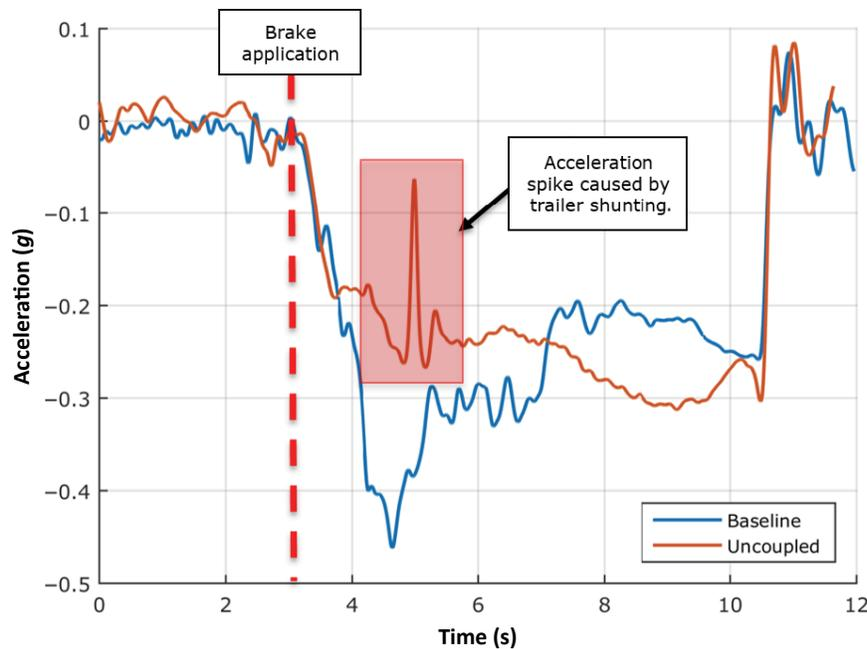
FIGURE 6 Longitudinal acceleration of truck when braking from 60 km/h (37 mph).
