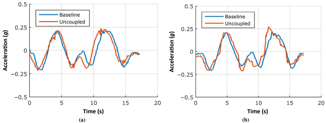
FIGURE 7 Lateral accelerations for (a) truck and (b) trailer at 60 km/h (37 mph).
