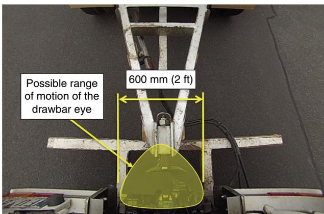
FIGURE 3 Observed possible range of motion of the drawbar eye.
