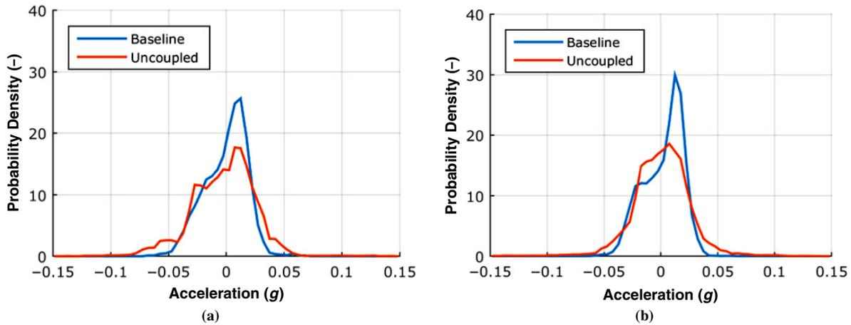
FIGURE 4 Probability density functions of longitudinal accelerations for (a) truck and (b) trailer at 80 km/h (50 mph).
