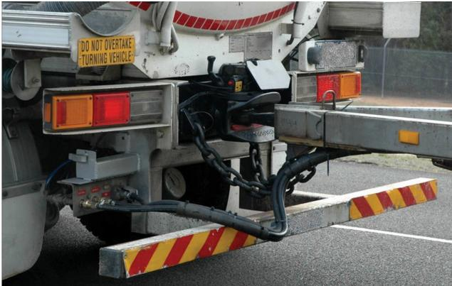
FIGURE 2 Pin coupling, release mechanism, and safety chain arrangement.
