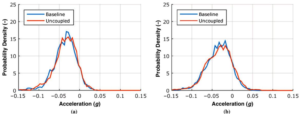
FIGURE 5 Probability density functions of lateral accelerations for (a) truck and (b) trailer at 80 km/h (50 mph).
