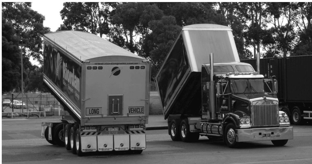
Figure 1 – A 3-axle Truck and 5-axle Dog Trailer Demonstrating Manoeuvrability and Tipping Both Bins Simultaneously
