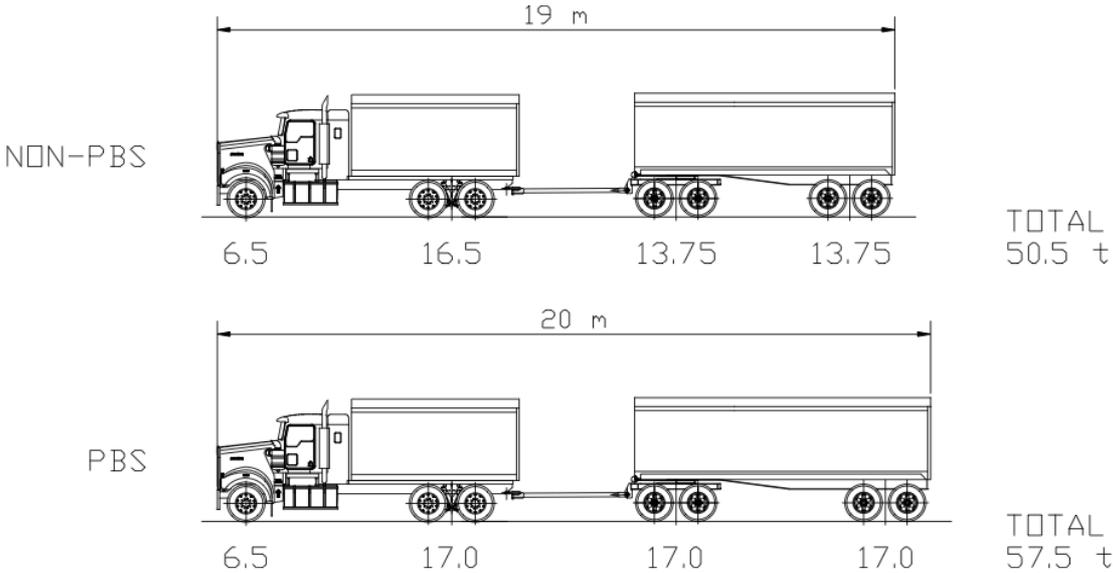
**Figure 3 – Difference between non-PBS and PBS truck and dog**
