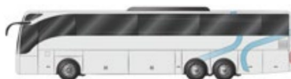
Figure 1. Three-axle bus with a dual-tyred drive axle and single-tyred tag axle
